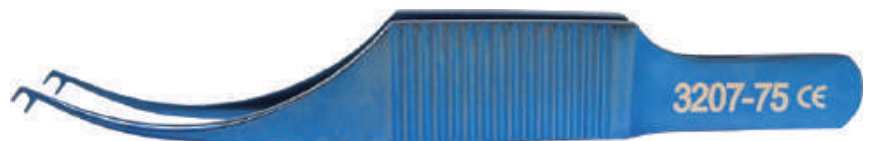
Polack Corneal Suturing Forceps, Colibri Style 3207-75 2.75mm tips, 1mm spread, 1 x 2 teeth, 75mm length
